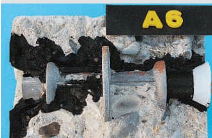
Shrinkage crack formation endangers the water impermeability with waterstop centre pieces ...
