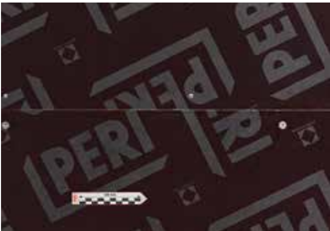
Formlining: film-coated plywood (phenolic resin) PERI Fin-Ply, smooth surface, very poor absorbency.
