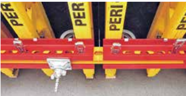
An offset of the panels at the joint up to 5 mm can be eliminated through the use of the Coupling VKS.
