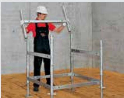
The stacking frame weighs less than 7 kg which facilitates ergonomic and fast assembly.
